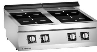
Electric range with pyroceram surface with AISI 304 stainless steel structure, 20/10 mm thickness top. Cooking surface in pyroceram, flush with worktop and sealed. Induction heating. 4 cooking independent areas. Kettle recognition sensors and automatic check devices. Forced cooling of electronic components. By the electromagnetic induction, pots (minimum Ø 120 mm) of suitable material are required.
