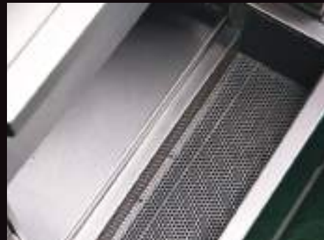
WASH TANK FILTER
