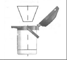
3 Place the airpot under the brewer against the airpot dispenser Locator (if featured). Align the center of the airpot Drip-Through with the outlet of the brewbasket.
