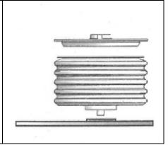
3 Carefully remove the bellows Cap.
